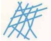
Thermo-softening plastics - No cross-links between the chains or carbon atoms.
