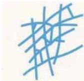
Thermosetting plastics - Cross-links between chain of carbon atoms.
